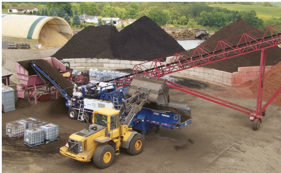
WOODBED offers five different types of colored enhanced mulches. Primary grind material is loaded into Peterson 4700B by Volvo L110E loader to be reground into a higher quality material before being colored in an Amerimulch system. Colored material then travels up the 100’ radial stacker to be dropped into conical piles for drying.
