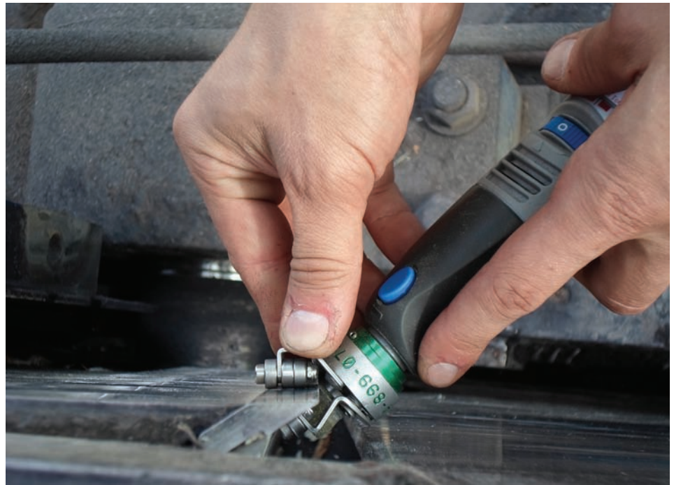
The Bevel Buddy™ sharpeners work very well with disc and drum style chippers and conventional pocket style, face mounted, and reversible/disposable knife systems. Sharpening knives with the Bevel Buddy takes a mere five minutes from shutting down the machine to starting it back up, according to Bob DeLullo.
